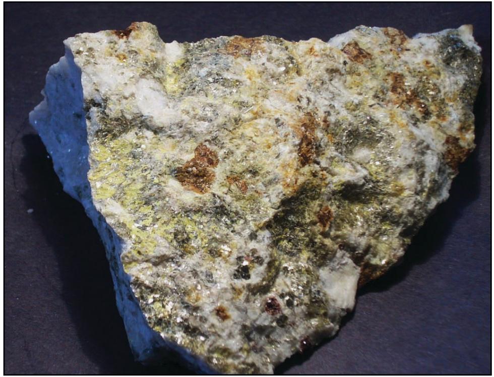
Figure 5.9: A portion of a feldspar-rich pegmatite from Pine Mountain Mine in Mitchell County, North Carolina, with inclusions of muscovite mica and garnet. Specimen is 13 centimeters (5 inches) wide.
