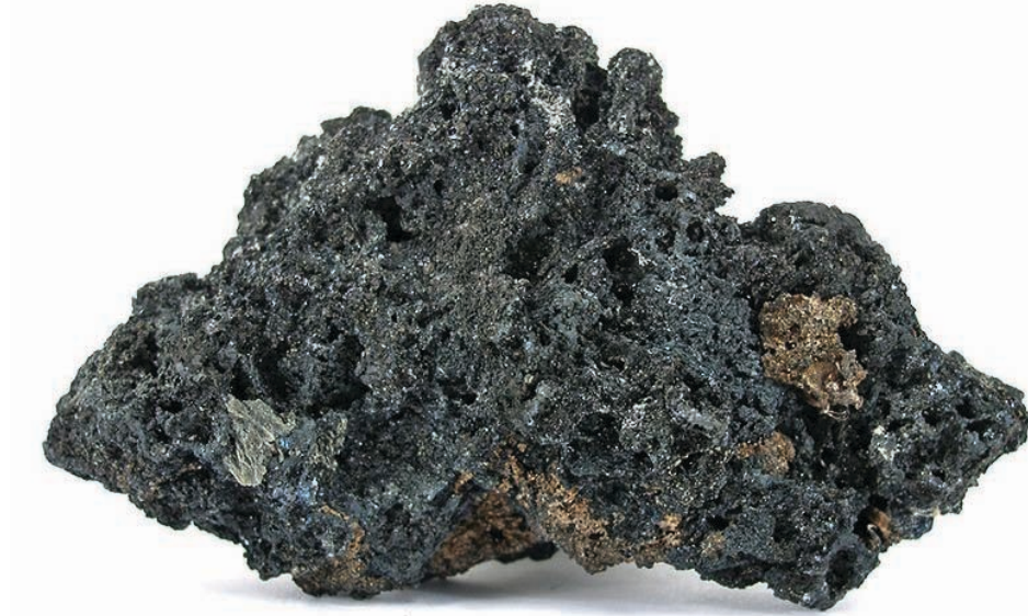
Figure 5.5: A lead-rich ore with patches of silver, from the Silver Hill Mine in the Carolina Slate Belt, Davidson County, North Carolina. Specimen is 8.8 centimeters (3.5 inches) wide.
