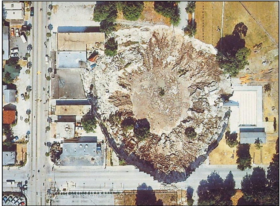
Figure 9.18: This 100-meter-wide (320-foot-wide) sinkhole formed in Winter Park, Florida, in 1981. It swallowed 190,000 cubic meters (250,000 cubic yards) of earth as well as vehicles and buildings. Today, it has been filled with water and is called Lake Rose.
