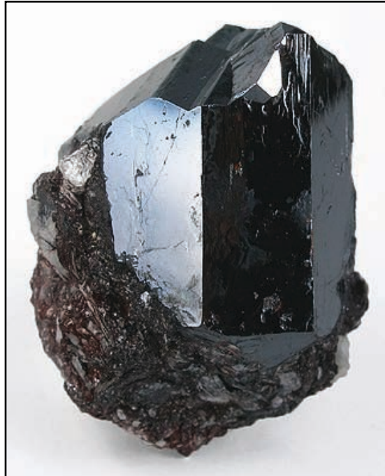
Figure 5.2: A crystal of rutile, composed primarily of titanium dioxide ( TiO_2 ). Although it appears dark in color, when powdered it becomes a brilliant white. Specimen is 4.4 centimeters (1.7 inches) in width.
