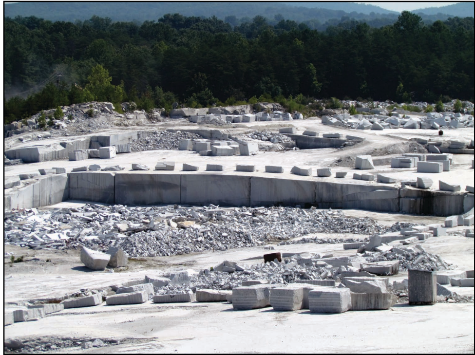
Figure 5.11: The open-faced granite quarry at Mt. Airy, North Carolina, produces over 610,000 meters (2 million feet) of white granite each year for use in construction and facing. The quarry was opened in 1743, and covers an area of roughly 372,000 square meters (4 million square feet).
