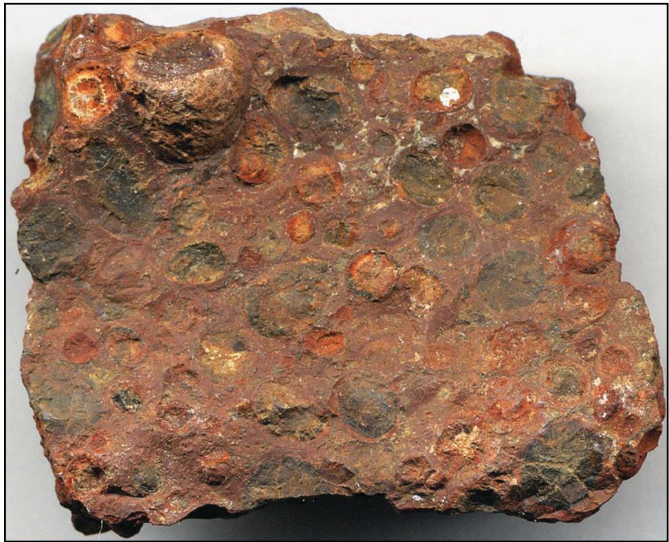
Figure 5.21: Bauxite is a rich aluminum ore, and the world's main source of aluminum. Specimen is 4.1 centimeters (1.6 inches) wide.
