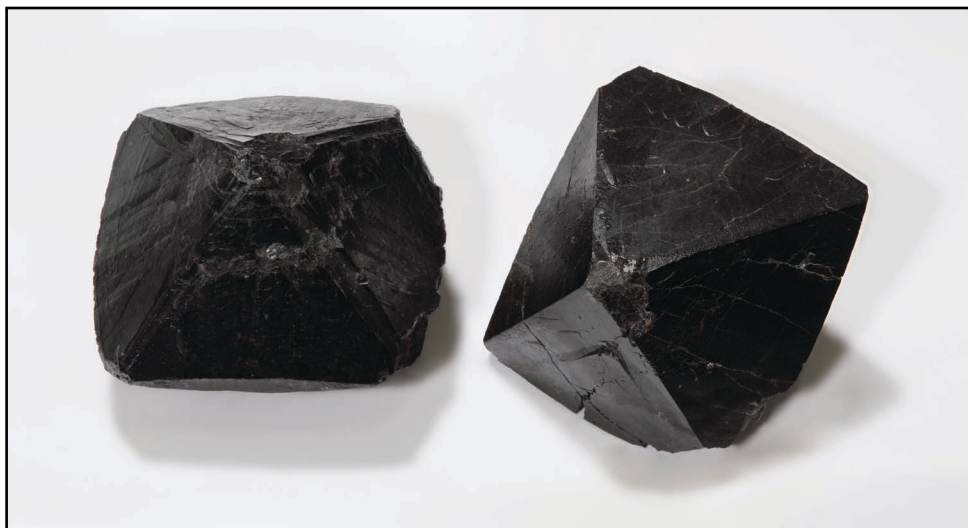
Figure 5.7: Bipyramidal crystals of cassiterite ( \text{SnO}_2 , tin oxide). Each crystal in the photo is approximately 30 millimeters (1.1 inches) across.
