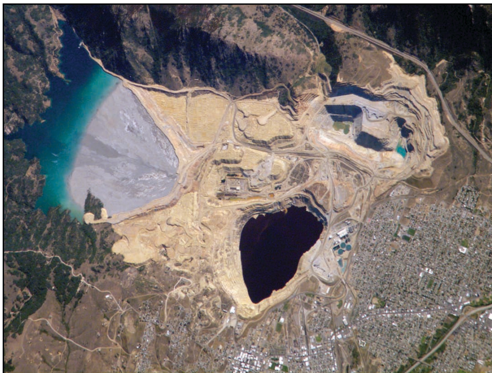
Figure 5.11: The Berkeley Pit and associated tailings pond. This open pit copper mine reaches a depth of about 540 meters (1780 feet), and is filled to a depth of about 270 meters (900 feet) with metal-laden acidic water. The mine is 1.6 kilometers (1 mile) long and 0.8 kilometers (0.5 miles) wide.
