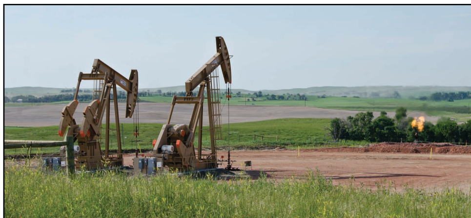
Figure 7.9: Oil pumpjacks in McKenzie County, North Dakota. The flame on the right-hand side is a flare that burns off natural gas separated from the oil.
